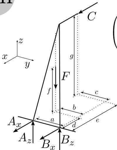
$$\begin{pmatrix} 0 \\ -a \\ 0 \end{pmatrix} \times \begin{pmatrix} A_x \\ 0 \\ A_z \end{pmatrix} + \begin{pmatrix} -d \\ -b \\ f \end{pmatrix} \times \begin{pmatrix} 0 \\ 0 \\ -F \end{pmatrix} + \begin{pmatrix} -e \\ -c \\ g \end{pmatrix} \times \begin{pmatrix} C \\ 0 \\ 0 \end{pmatrix} = 0$$
