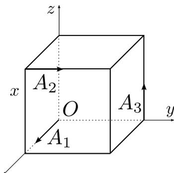
$$\vec{R} = \sum_i A_i, \vec{M} = \begin{pmatrix} a \\ 0 \\ a \end{pmatrix} \times \begin{pmatrix} 0 \\ A \\ 0 \end{pmatrix} + \begin{pmatrix} 0 \\ a \\ 0 \end{pmatrix} \times \begin{pmatrix} 0 \\ 0 \\ A \end{pmatrix}$$
